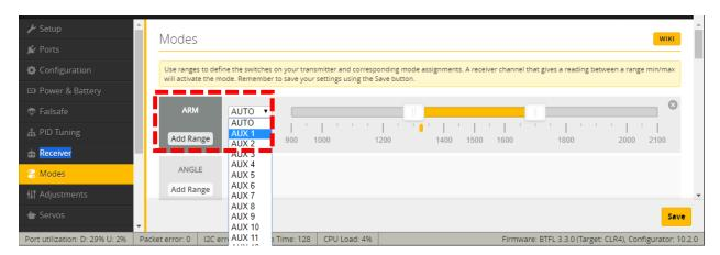
3. Turn on your transmitter. Plug in a LiPo. The small yellow indicator will move to indicate the current position of the Aux1 channel.
