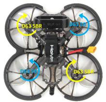
The default motor directions for a Cleanflight or Betaflight quadcopter are shown to the left. Based on this, the correct way to install the props is as shown.
